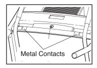
is detected, the heart symbol in the display will begin to flash, one or two dashes will appear, and then your heart rate will be shown. For the most accurate heart rate reading, continue to hold the contacts for about 15 seconds.
